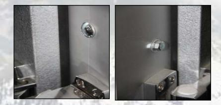
DO NOT OVER COMPRESS GASKET! If the gasket is not sealing without over compressing the gasket, the casings are out of plane.
